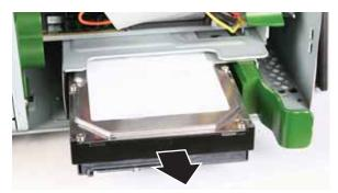
5 Make sure the hard drive release lever is still fully extended, then slide the new hard drive all the way into the hard drive bay by pushing on the hard drive itself (not the lever). Make sure that you slide the drive in until it is flush with the edge of the hard drive bay.
